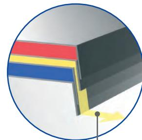
*Leaks escape into the atmosphere through the air gap between the double walls.*
