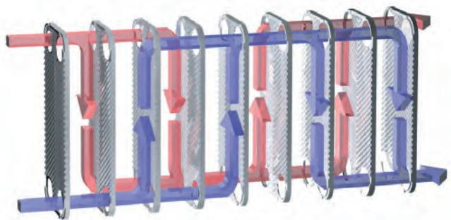
multi-pass - system of channels is divided into groups which are connected in series.
