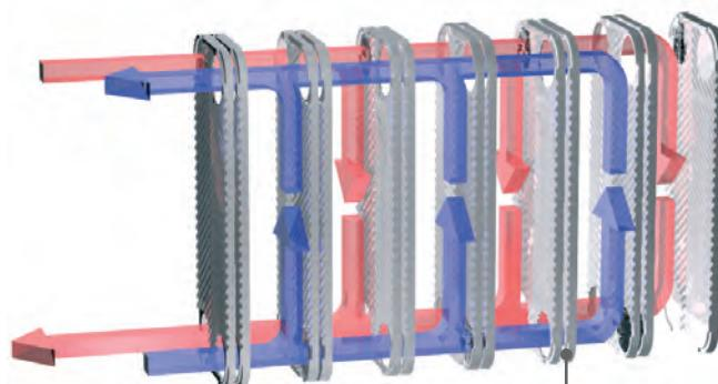
*Double walls allow leaks to be visually detected without cross contaminating the fluid streams.*
